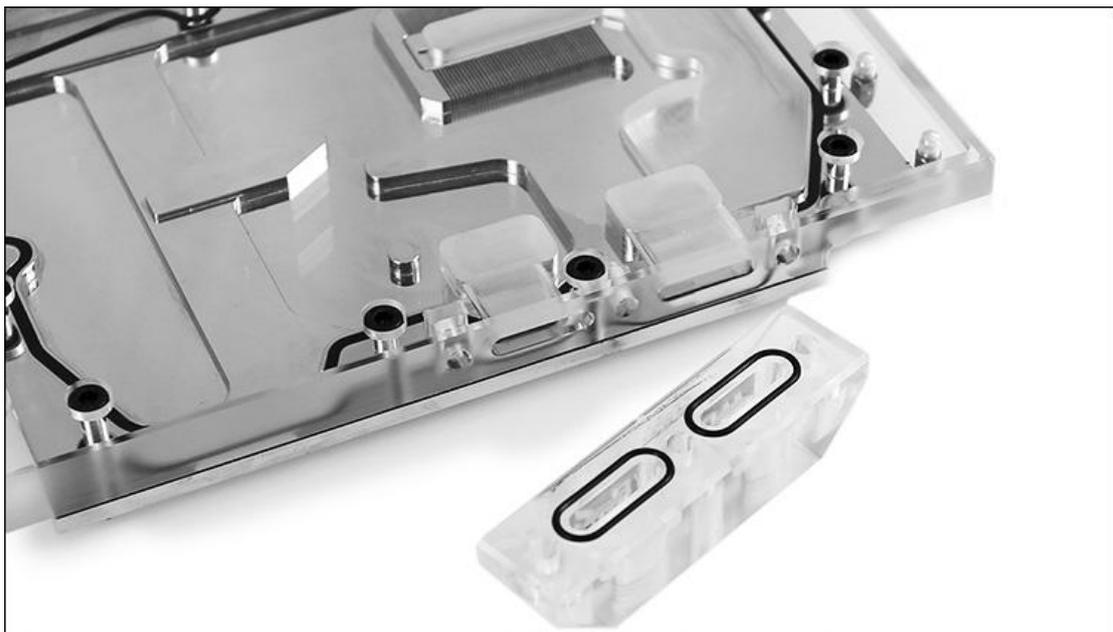
Press the seal ring in the rubber ring slot of the terminal connector
