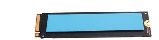
2.Apply thermal grease to one side of the hard disk drive
