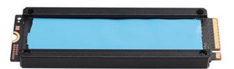
4.Apply thermal grease on the other side (In the case of a hard disk drive with a chip on both sides, select one side to apply the 0.5mm gray gasket)
