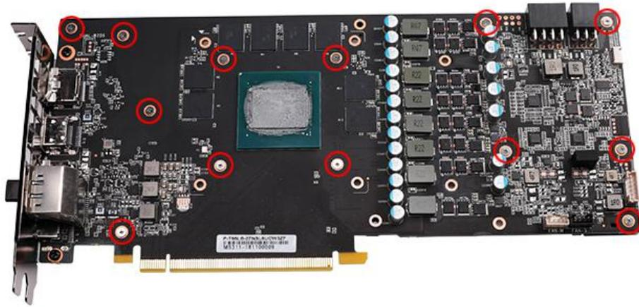
2.Remove the red position screws in the picture
