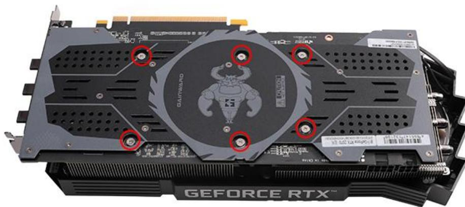
1.Remove the red position screws in the picture
