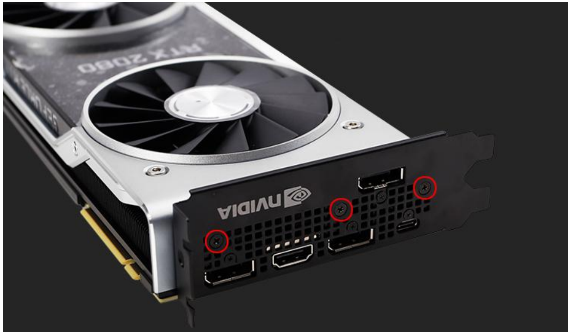
2.Remove the screws in the mark red position as shown
